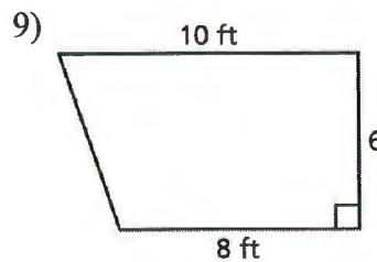
$$\begin{aligned} A &= \frac{1}{2}(b_1 + b_2)h \\ &= \frac{1}{2}(10 + 8)6 \\ &= \frac{1}{2}(18)6 \\ &= \frac{1}{2} \cdot 108 \\ &= 54 \text{ ft}^2 \end{aligned}$$
