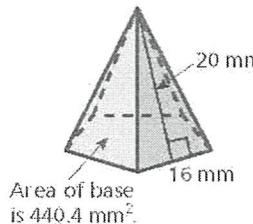
$$\begin{aligned} SA &= 5\left(\frac{1}{2} \cdot 16 \cdot 20\right) + 440.4 \\ &= 5(160) + 440.4 \\ &= 800 + 440.4 \\ &= \boxed{1240.4 \text{ mm}^2} \end{aligned}$$
